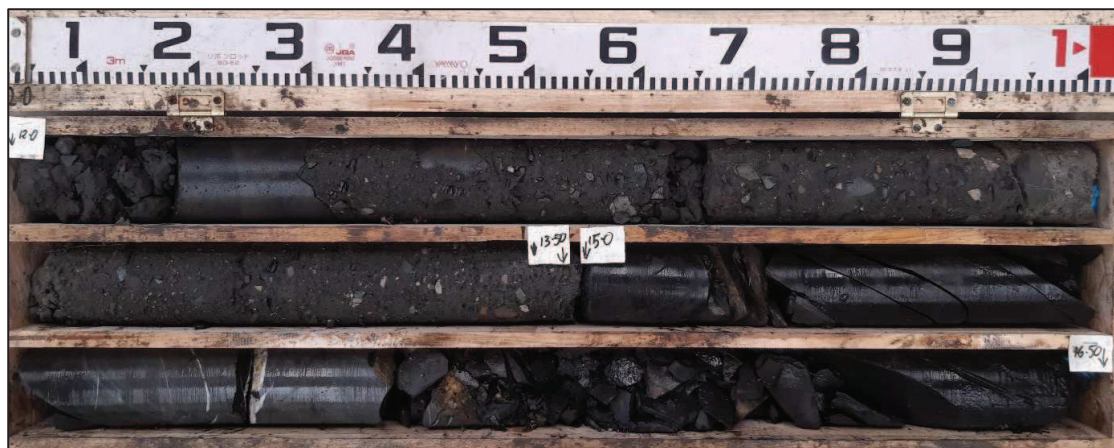
Photo 3 – Core recovery of glacial till and bedrock at RC09 (12.0 to 16.5 m BGL)
